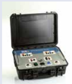
20A DC BOOSTER FOR WINDING RESISTANCE TEST
