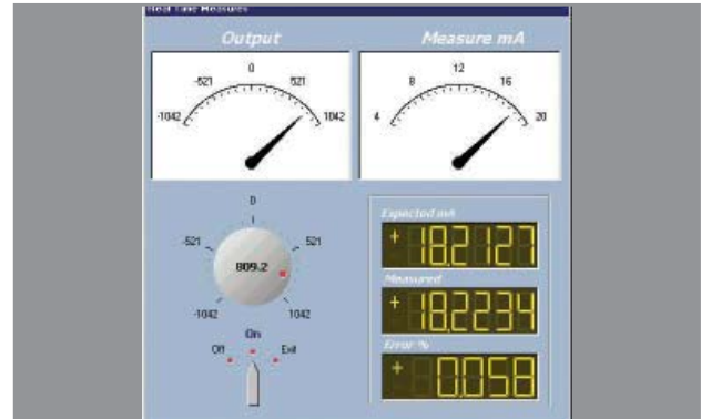
Transducer Test Program manual control
