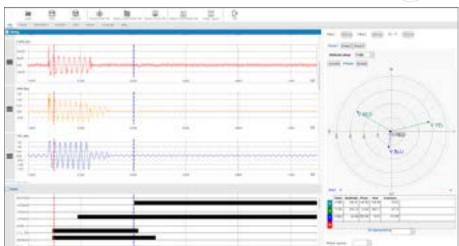
The Playback Waveform module is used for the accurate representation and reproduction of files containing the recording of a real fault event. In this way it is possible to verify the correct or incorrect behavior of the protective relay.
